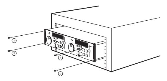
The player will operate properly when the main unit is mounted with the front panel at an angle within 15 degrees of the vertical plane. If the unit is tilted excessively, discs may not load or unload properly.
