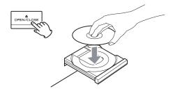
Press the OPEN/CLOSE (**△**) button, place a disc on the disc tray with the disc label side up, and then press the OPEN/CLOSE (**△**) button to close the disc tray.
