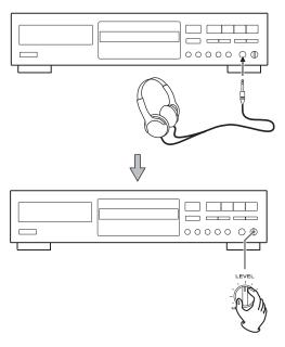
For private listening, first reduce the volume level to minimum. Then insert the plug from your headphones into the PHONES jack, and adjust the volume by turning the LEVEL knob.
