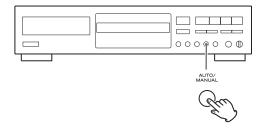
When the AUTO/MANUAL button is pressed once, the current increment level is displayed. Press the AUTO/MANUAL button repeatedly to select another setting.
