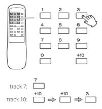
The selected track is programmed. To program more than one track, press the numbers subsequently.
