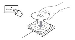
Press the OPEN/CLOSE (♠) button, place a disc on the disc tray with the disc label side up, and then press the OPEN/CLOSE (♠) button to close the disc tray.
