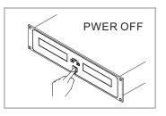
Switch off the power after the disc holder has been closed with the OPEN/CLOSE button.
