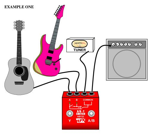
• Example One shows the ABY32 selecting between two instruments to a single amplifer.
