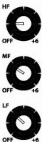
EQ is used to boost and cut specific frequencies. The Xone:DX features 3-band EQ with low, mid and high frequency controls. The knobs go from full cut (or kill) when turned all the way left, unity when facing straight up, and +6 dB of boost when turned all the way to the right.
