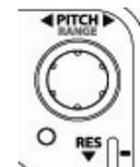
The playback speed of the track is controlled by the PITCH knob. By default the knob is set to fine tune pitch adjustments, and turning the knob anti-clockwise will slow the track down, turning it clockwise will speed the track up. Pressing and holding the PITCH knob down will allow you to make coarse (big) pitch adjustments.
