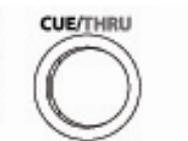
When CUE is pressed on a track, the audio is sent into the headphones so that you can cue the track without it appearing in the main mix. The headphone LEVEL knob controls the headphone volume.
