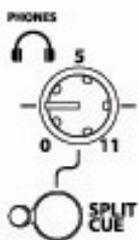
**PHONES LEVEL CONTROL** - adjusts the level of the signal sent to the headphones. The headphones can be connected to the Xone:DX via 1/4 inch and 3.5mm Jack sockets.
