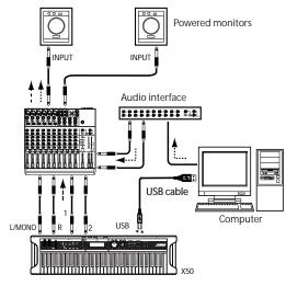
If you want to apply a plug-in effect to the X50's audio signals, or to control the X50's audio signals in your host application together with the audio data from the KORG Legacy Collection or other audio tracks, make connections as shown below. Make settings as appropriate for the host application you're using.
