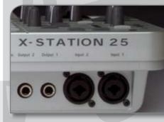
Fully featured 24-bit audio interface with phantom power and digital out (S/PDIF)
