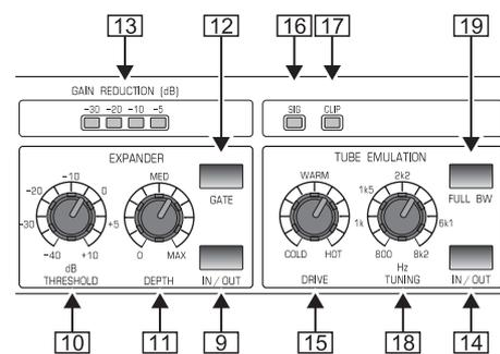
Fig. 2.2: Expander and tube emulation
