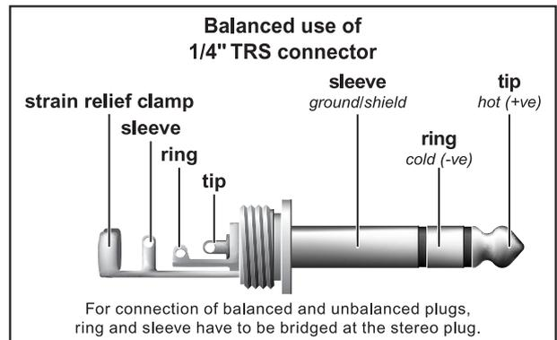
Fig. 7.3: 1/4" stereo jack connector
