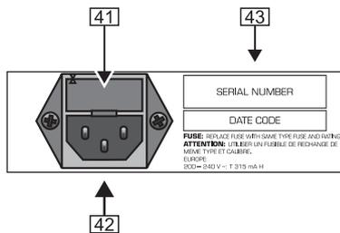
Fig. 2.6: Mains connector and fuse holder
