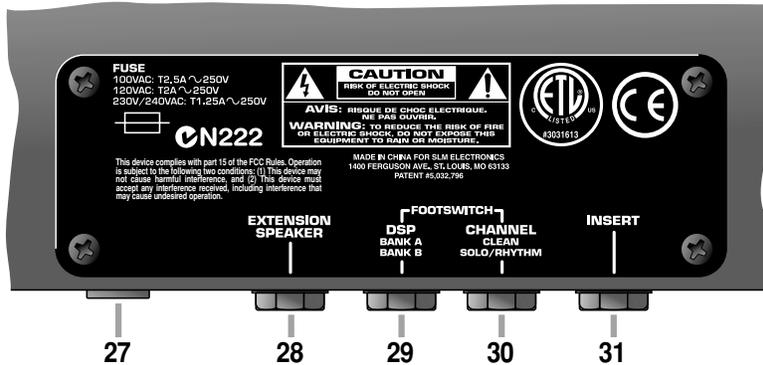
**27: FUSE:** The fuse protects the amplifier from damages caused by a faulty AC power source and/or other problems. If the fuse opens, replace it **ONLY** with the same size and type. If fuses continue to fail, check the AC source – if the source is okay, contact your Crate dealer for service information.
