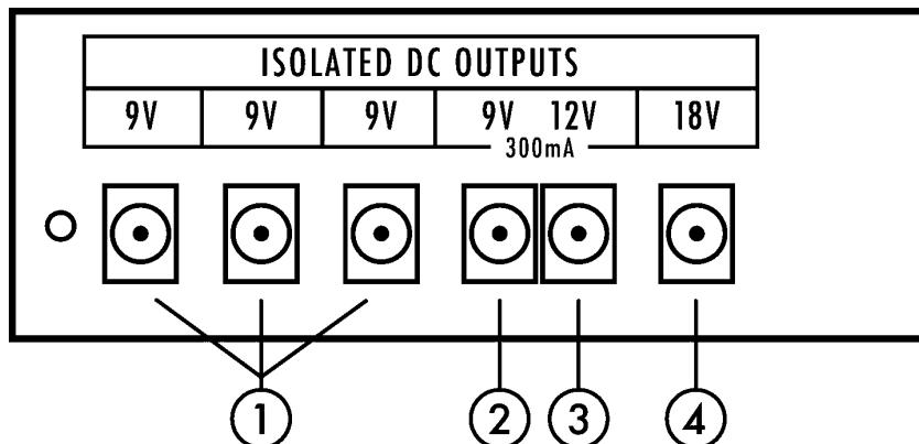
1) 9V outputs (3). Use for all ordinary pedals which operate from a 9V battery or require less than 100mA.
