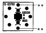
Place the top panel and fix it with four screws. Then replace each fader knob.
