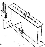
•Insert the connector to the new fader unit.
