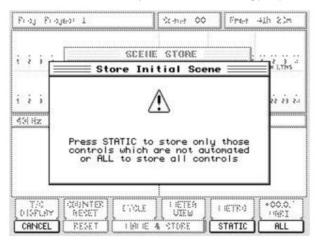
As the prompt suggests, you can select to store all mixer settings - i.e. automated controls (faders, pans, FX sends, channel on/off) and 'static' controls (EQ) - or just 'static' controls.
