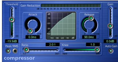
The Compressor tightens up the dynamics of a signal by lowering the volume when it rises above a certain level, called the *Threshold*. This decreases the difference between the softest and loudest parts of the music, increasing the perceived volume. This can give the sound more focus, by making the key parts stand out while preventing the accompanying parts from becoming lost or inaudible.
