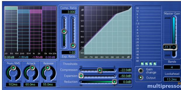
The Multipressor (short for *multiband compressor*) is used as a mastering tool in many different situations. The Multipressor splits the incoming signal into two to four different frequency bands, each of which is compressed independently. This permits higher levels of compression without producing a pumping effect.
