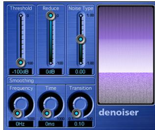
You can eliminate or reduce many kinds of low-level noise (noise floor) from an audio signal with the Denoiser. The main parameters of the Denoiser are *Threshold*, *Reduce*, and *Noise Type*. The Threshold parameter determines the level below which signals are interpreted as noise floor. The recommended method for setting the Threshold is to find a passage where only noise is audible, then set the Threshold so that signals at this volume level are filtered out.
