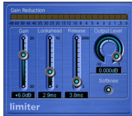
The Limiter prevents the audio signal from exceeding a maximum volume level. While a compressor gradually lowers levels above a threshold, the Limiter uses a fixed limit at 0 dB. The Limiter can help increase the perceived loudness without clipping. This is achieved by raising the input level against the fixed 0 dB limit with the *Gain* parameter.
