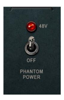
**Phantom power switch** – by default switched on when you're loading a Mic Emulation in the Discrete 4 and Discrete 8 Control Panel.
