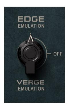
**Mode switch** – allows you to switch between Verge, Edge or turn the emulation off.
