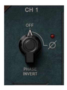
**Phase invert** – allows you to invert the polar pattern of the signal in the selected Mic input.
