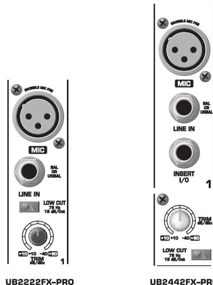
Fig. 2.1: Connectors and controls of mic/line inputs
