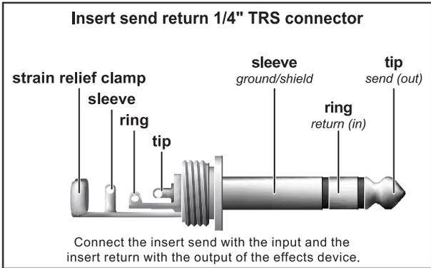
Connect the insert send with the input and the insert return with the output of the effects device.
