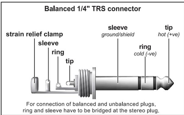
For connection of balanced and unbalanced plugs, ring and sleeve have to be bridged at the stereo plug.
