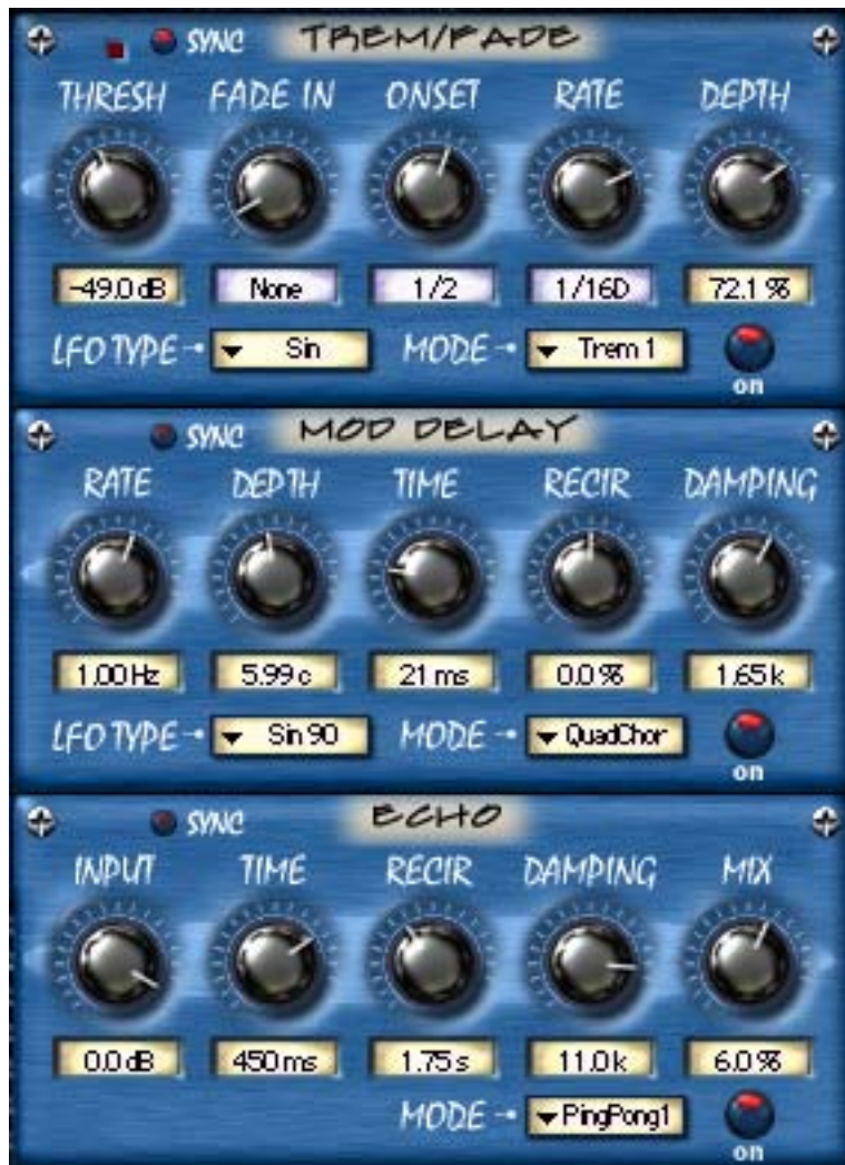
Figure 145. The TremModEcho plug-in contains three modules
