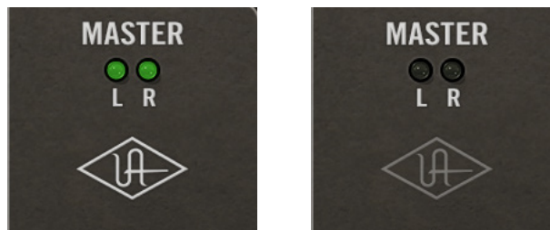
Power switch active (left) and powered off (right).
