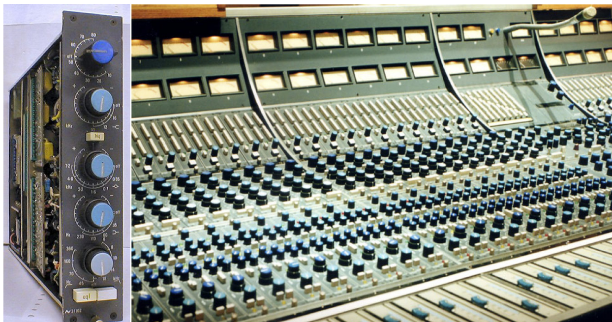
One Neve 31102 EQ hardware module (left) and 31102s installed in a Neve 8068 console
