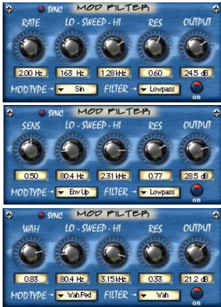
Figure 142. The Mod Filter plug-in window The label and function of the first knob depends upon the Mod Type menu selection.
