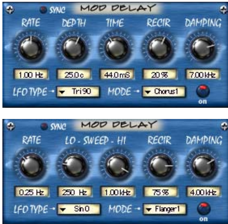
Figure 145. The Mod Delay module The label and function of the second two knobs depend upon the Mode menu selection.
