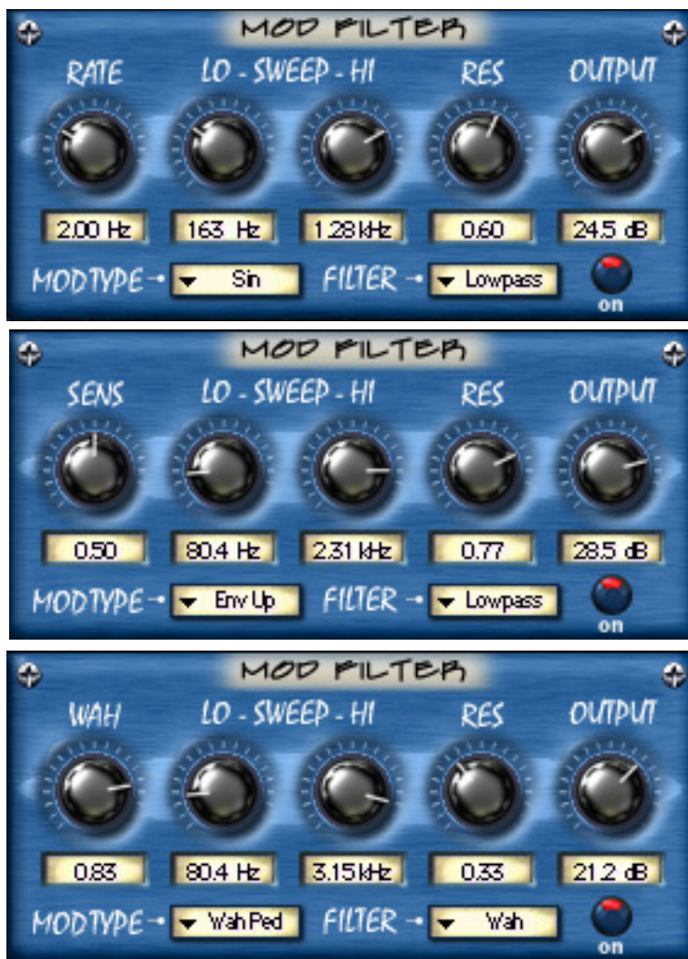
Figure 45. The Mod Filter plugin window The label and function of the first knob depends upon the Mod Type menu selection.
