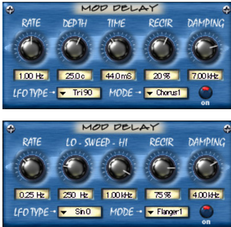
Figure 48. The Mod Delay module The label and function of the second two knobs depend upon the Mode menu selection.
