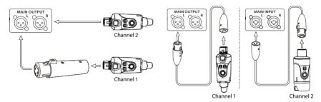
If the XLR inputs/outputs on your mixer are very close to each other, using the XLR adapter with a Transmitter allows you to plug in two Transmitters side-by-side. Using an XLR cable (not included) as an extension for a Transmitter allows you to connect the components to a mixer where the inputs/outputs are very close together. It can also resolve wireless signal interference issues if you have too many wireless units in the area.
