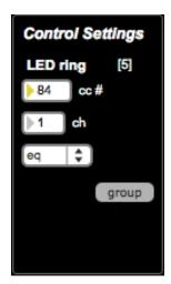
The LED rings for the encoders can be controlled independently of the encoder value. This is useful if you want to use the rings to display an absolute value while the encoders are in relative mode.
