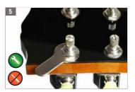
Use the wrench that comes with the set to tighten the Hex Nuts of the RoboHeads.
