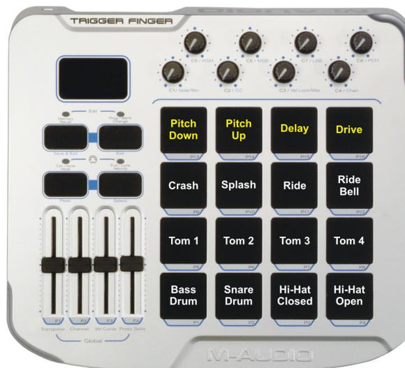
The yellow labels indicate pads that are not transmitting MIDI note data—they're only sending MIDI controller messages. These messages are being used to control the pitch of the kit, the reverb send, and the drive of a distortion plug-in.
