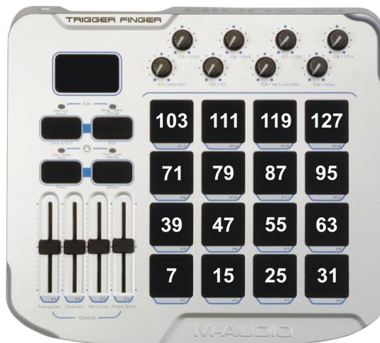
*When using one of the Spread Presets, each pad has the Velocity Lock value shown here.*
