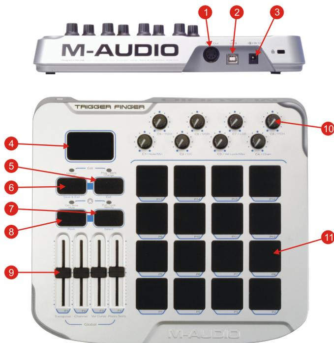
1. **MIDI Out Jack:** This jack outputs MIDI information from either the Trigger Finger control surface or from the host computer.
