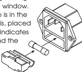
Check also the fuse ratings to ensure they match the ratings indicated on the rear panel.
