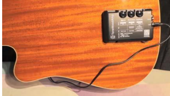
Figure C-3 Neo-D pickup cable plugged into ToneWoodAmp
