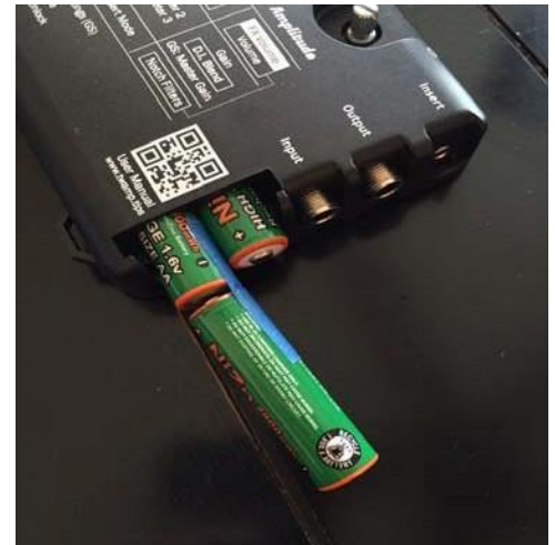
Figure B-1 Taping two rechargeable batteries together for easy insertion and removal
