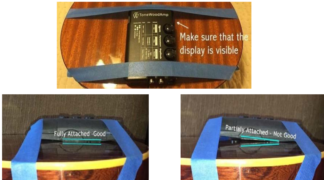
Figure 2-3 ToneWoodAmp taped in position for testing
