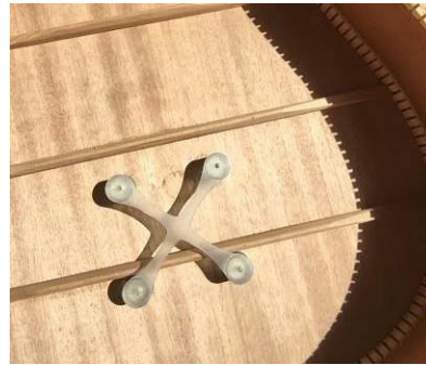
Figure 2-5 Magnetic x-brace alone (left) and inside the guitar (right)
