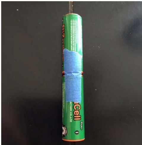
Figure B-1 Taping two rechargeable batteries together for easy insertion and removal
