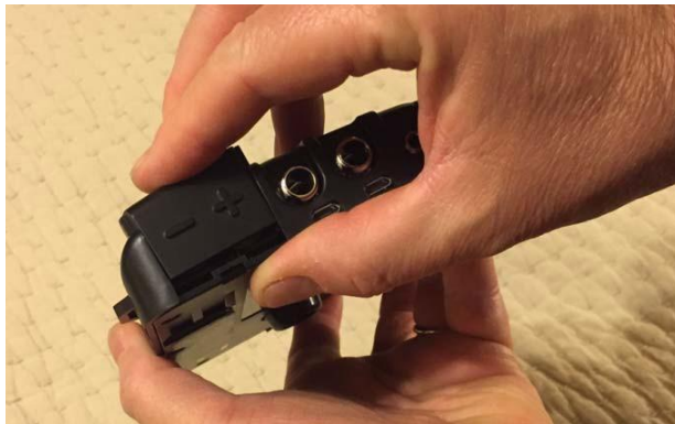
Figure 2-1 Removal of battery door (left), and proper polarity of batteries (right)
