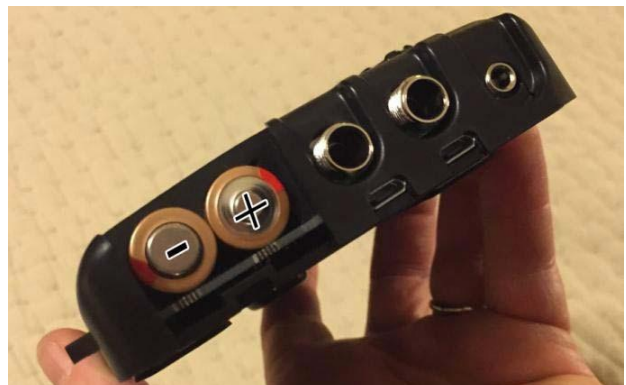
Figure 2-1 Removal of battery door (left), and proper polarity of batteries (right)
