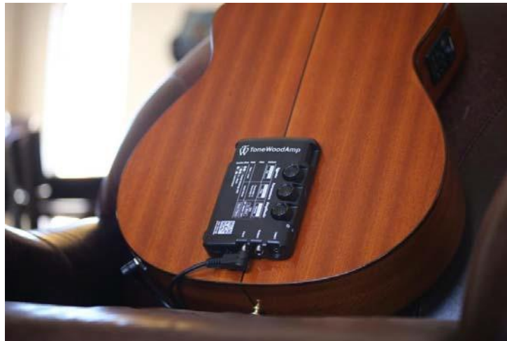
Figure 2-6 ToneWoodAmp mounted on back of guitar
