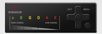
TRONICAL TUNE HAS A SUPERIOR DYNAMIC RANGE TO SENSE THE SOLID-BORNE SOUND OF YOUR INSTRUMENT (>130DB). THIS IS ACHIEVED BY A PIEZO TRANSDUCER, A DYNAMICAL ADJUSTABLE AMPLIFIER AND A 24 ANALOG TO DIGITAL CONVERTER (ADC). WITH THE "GAIN SETTING" THE STARTING POINT OF THE AMPLIFIER IS SET. FROM THIS STARTING POINT THE AMPLIFIER IS ADJUSTED DURING THE TUNING PROCESS IN THE RANGE OF +-9DB.
