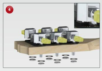
MAKE SURE THAT ALL PCB DRILL HOLES ARE IN ALIGNMENT WITH THE NECK'S TUNER HOLES. PUT THE ROBOHEADS THROUGH THE RESPECTIVE HOLES. MOUNT THE HEX-NUTS.
