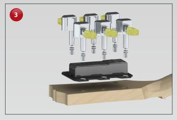
PLACE THE CONTACTING PCB ON THE NECK OF THE GUITAR, THE BATTERY COMPARTMENT HAS TO FACE TOWARDS THE TOP OF THE HEADSTOCK.
