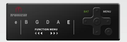
**PUSH "ON"** button. The system activates with the last completed tuning in MULTI-STRING MODE.
