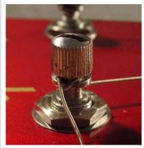
TIGHTEN WITH A SMALL COIN THE LOCK NUT SMOOTHLY BY HAND. THE STRING MUST ENCIRCLE THE STRING SHAFT COMPLETELY.
