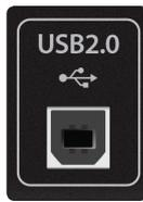
**USB 2.0 port.** Use this port to connect your StudioLive AR-series mixer to a USB port on your computer when using the mixer as an audio interface. *See your StudioLive AR-series Software Reference Manual* for further information.
