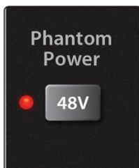
**48-volt Phantom Power.** The StudioLive AR mixers provide global 48V phantom power for all microphone inputs.
