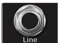
**Line-level Inputs.** Each channel of your StudioLive AR-series mixer has a 1/4-inch, balanced TRS connection for line-level input. Typical examples of line-level connections are synthesizer outputs, CD/DVD-player outputs, and (with exceptions) signal-processor inputs and outputs.
