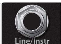
**Instrument Inputs.** Channels 1 and 2 are equipped with an input that can be switched between line and instrument. Use these 1/4-inch connections for instruments that don't have internal preamps (guitar, bass, etc.). **See Input Source button in Section 3.2 for more information.**
