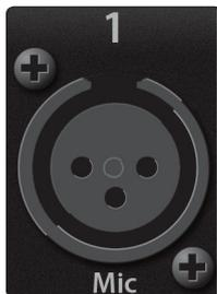
**Microphone Inputs.** Your StudioLive AR-series mixer is equipped with high-quality microphone preamplifiers for use with all types of microphones.
