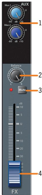
The internal FX return allows you to adjust the amount of the effects output you would like in your main and monitor mixes.
