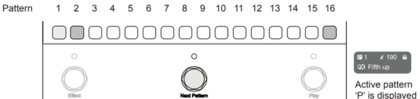
+  Copying a Pattern: In Song View, Keep Hold [Pad] for the Source to copy until it turns blue, then Press [Pad] for the destination to paste the pattern. Then release holding the first pad.
