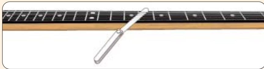
Figure C. Measuring relief with feeler gauge
