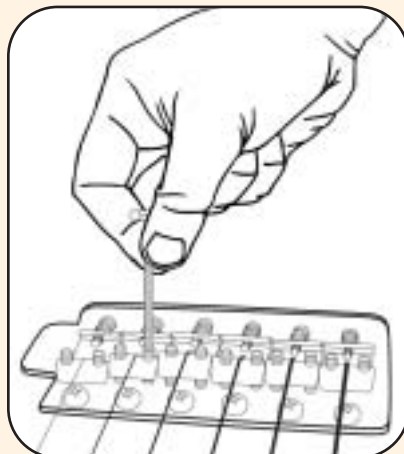
Figure F. (Electric Guitar saddle height adjustment)
