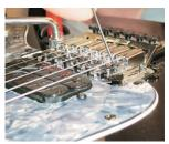
Using a 1.5mm Allen wrench and the range tuner set screw, tune your guitar to any tuning you desire. You can increase the pitch of a given string by turning the set screw clockwise, and decrease the pitch of the string by turning the set screw counterclockwise. (Remember not to use the fine tuner screws for this tuning.)
