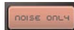
Noise Only mode allows you to hear just what’s being removed from an audio signal
