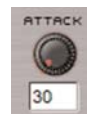
The Noise Gate’s Attack can be adjusted with a knob, or by entering a number
