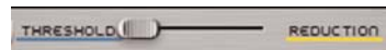
The Threshold/Reduction Control slider allows viewing just Threshold sliders, just Reduction sliders, or a percentage of both simultaneously
