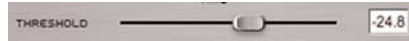
The Noise Gate’s Threshold can be adjusted with a slider, or by entering a numerical value
