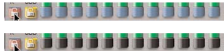
Above: All Threshold sliders locked together – they move together Below: All Threshold sliders unlocked – they now move independently
