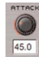
The Attack knob controls how fast broadband noise reduction is turned on
