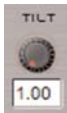
The Release Tilt knob varies the ratio of Release values between low and high frequency bands
