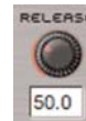
The Release knob controls how fast broadband noise reduction is turned off
