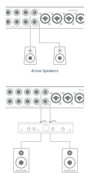
All the line output connectors are 3-pole (TRS) ¼" (6.35 mm) jack sockets, and are electronically balanced. Typical consumer (hi-fi) amplifiers and small powered monitors will probably have unbalanced inputs, either on phono (RCA) sockets, or via a 3.5 mm 3-pole jack plug intended for direct connection to a computer. In either case, use a suitable connecting cable with jack plugs at one end.
