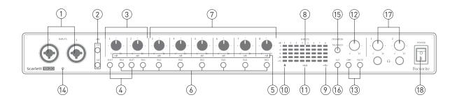
The front panel includes all the input gain and monitoring controls as well as two of the input connectors for Mic, Line and Instrument signals.
