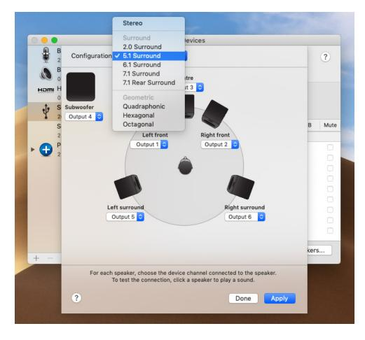
The example below shows how you would connect the six loudspeakers in a 5.1 surround monitoring arrangement.
