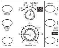
Look for the illuminated LOW BAND INDICATOR LED over the first GAIN control. Now, adjust the first gain
