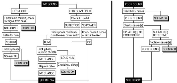
If the problem isn't covered above, or if the steps lead you here, then contact your Ampeg dealer for service information. Also, you should refer your amp for servicing if it gets dropped, has liquid spilled into it, or sustains damage to its power cord (see page 2). Regular maintenance and cleaning should be performed on a routine basis to prolong the amplifier's useful life.
