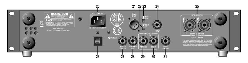
**20. AC LINE IN:** Firmly insert the supplied AC power cord into this socket until it is fully seated. Plug the male end of the cord into a grounded AC outlet. *DO NOT DEFEAT THE GROUND PRONG OF THE AC PLUG!*
