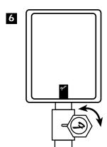
Loosen collar handknob and raise equipment to the desired height. Do not extend the center pole more than 36" (91.4 cm) above the locking collar support. Re-tighten handknob and check the stability of the unit at the desired height setting.
