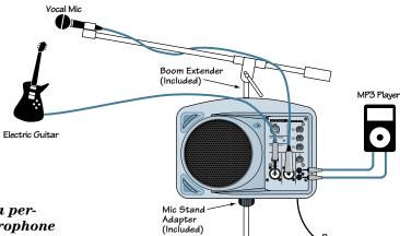
This illustrates how to use the SRM150 as a personal monitor. Mount the SRM150 on a microphone stand using the Mic Stand Mounting Bracket included with the SRM150. Attach the Boom Extender (also included) to the top of the SRM150 and use a microphone boom to hold your microphone.
