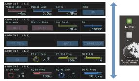
3. Turn the [F1]–[F4] knobs to edit the values, and then press the [F1]–[F4] knobs.
