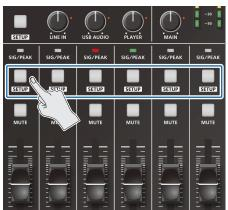
The parameter for the channel you pressed is shown in the parameter area.
