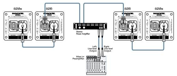
S218s AND S215: WITH A MIXER AND POWER AMPLIFIER, USING THE 1/4" THRU JACKS
