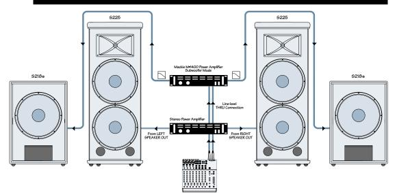
**Note:** The FR Series  $M \bullet 1400$  power amplifiers have a built-in subwoofer crossover. If you are not using a Mackie  $M \bullet 1400$  amplifier, you can use an active crossover between the first and second amplifiers with the crossover set between 125 Hz to 180 Hz. This allows more amplifier power for the low frequencies rather than being wasted as heat in the S218s' internal built-in crossover.
