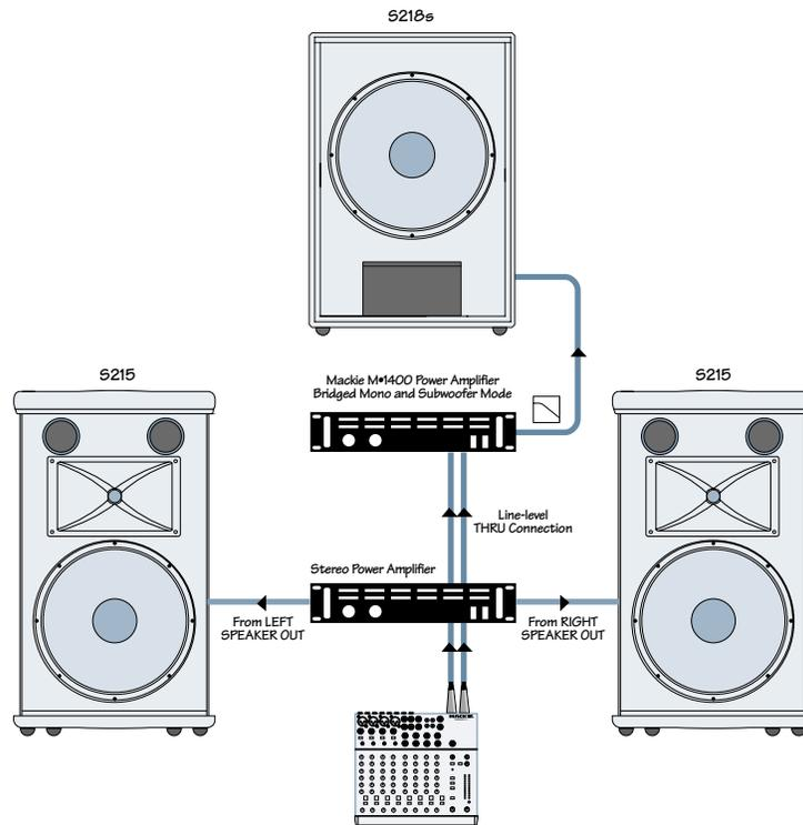
**Note:** The FR Series M•1400 power amplifiers have a built-in subwoofer crossover. If you are not using a Mackie M•1400 amplifier, you can use an active crossover between the first and second amplifiers with the crossover set between 125 Hz to 180 Hz. This allows more amplifier power for the low frequencies rather than being wasted as heat in the S218s' internal built-in crossover.
