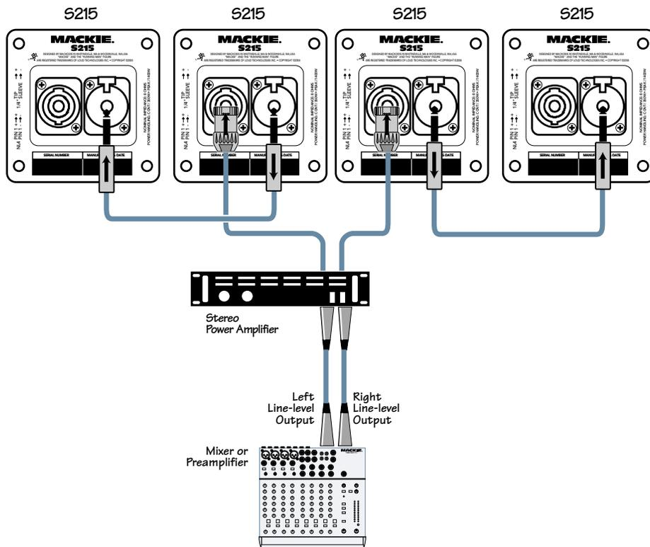
**S215: WITH A MIXER AND POWER AMPLIFIER, USING THE 1/4" THRU JACKS**
