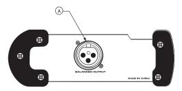
A BALANCED OUTPUT- XLR balanced connector outputs carrying the summed signal from Microphone 1 and 2.
