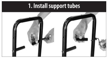
With the RocknRoller Multi-Cart extended and both handles raised, install the round support tubes. Insert the 5/16" low profile socket head screws into the handle's pre-drilled holes from the outer edge, so the support tube in inside the handle. Make sure each tube is set to the same height before screwing them in securely.
