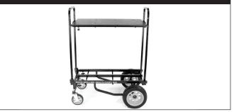
The shelf may also be used while the cart is compact. Simply replace the extension shelf with the short, hooked mounting brackets. The open end of hook should be facing downwards. Please make sure to secure the brackets by tightening the wing bolts firmly before installing the shelf.
