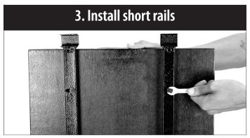
**Install the 2 short metal rails to the 18" x 16" extension shelf.** Position the rails on the board so the hooked end sits just past the same edge. Insert small Allen bolts into the shelf from the textured side, and secure with a washer and 10 mm hex nut. Do not tighten the bolts completely yet.
