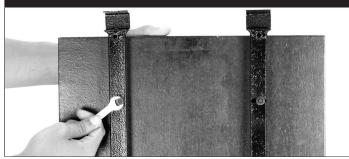
**Install the 2 long metal rails to the 32" x 16" main shelf.** Position the rails on the board so the hooked end sits just past the same edge. Insert small Allen bolts into the shelf from the textured side, and secure with a washer and 10 mm hex nut. Do not tighten the bolts completely yet.
