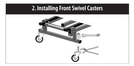
Attach front swivel casters as shown. While tightening lock nuts, grip bearing cap with channel lock pliers or pipe wrench to prevent threaded stem from turning. Tighten lock nuts firmly, but not excessively tight. Check lock nut tightness on caster stems periodically.
