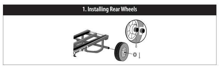
Gently slide wheel over axle as shown. Do not force wheels onto axle. It is recommended to lubricate axles with light grease before installing. Install cotter pins and bend ends outward.
