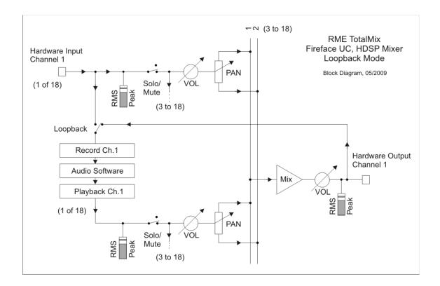
The block diagram shows how the software's input signal is played back, and fed back from the hardware output to the software input.
