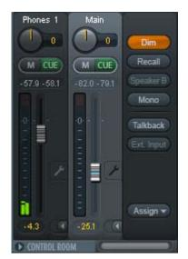
**Speaker B.** Switches playback from Main Out to Main Out B. The faders of the channels Main and Speaker B can be ganged via Link.
