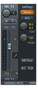
Width. Setting the stereo width. 1.00 equals full stereo, 0.00 mono, -1.00 swapped channels.
