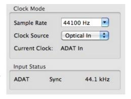
RME's exclusive **SyncCheck** technology (first implemented in the Hammerfall) enables an easy to use check and display of the current clock status. *Input Status* indicates whether there is a valid signal (Lock, No Lock) for each input (Word Clock, ADAT and SPDIF), or if there is a valid *and* synchronous signal (Sync). In the field *Clock Mode* the clock reference is shown (Current...). See chapter 31.1.
