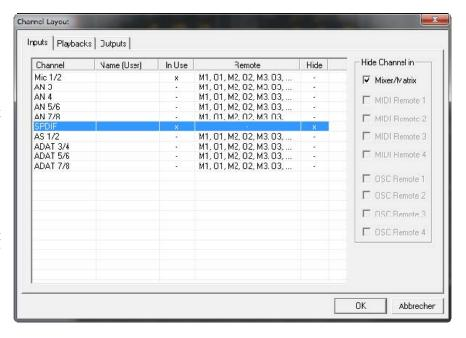
Rows Inputs, Playbacks and Outputs are set up individually by the tabs at the top. *In Use* shows which channels are currently used in the mixing process.
