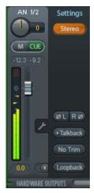
Another difference to the input and playback channels is the **Cue** button instead of Solo. A click on Cue sends the respective Hardware Output's audio to the **Main** Out, or any of the Phones outputs (option *Assign / Cue to* in the Control Room section). With this any hardware output can be controlled and listened to through the monitoring output very conveniently.
