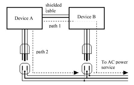
One path goes from device A to ground via the ground terminal of the three-conductor AC power cord, but A also sees a path to ground through the shielded cable and AC ground of device B. Because ground wires have a small amount of resistance, small amounts of current can flow through ground and generate a voltage along the cable shield. This signal may end up getting induced into the hot conductor.
