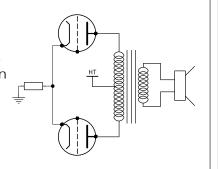
the use of a 12BH7 dual triode valve in push-pull configuration producing 5 Watts output, which is rich in valve harmonics and compression, sounding full and toneful even at the lowest volume level.
