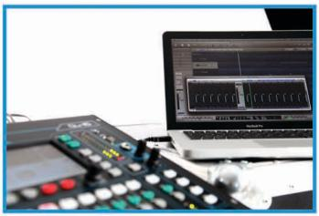
The returns from the computer can be assigned to the Input channels. The interface is class-compliant on Mac OS X – and drivers are available for Windows systems. Either way, it will be recognized straightaway by any DAW supporting ASIO or Core Audio, including Logic, Cubase, Reaper, and Pro Tools.
