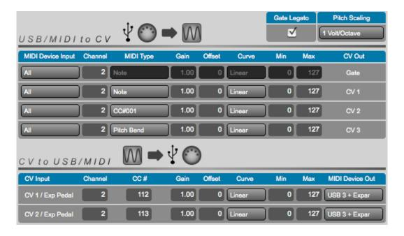
Here you can choose how the QuNexus keys send and receive CV (Control Voltage). QuNexus has 4 possible CV outputs and 2 possible CV inputs (see the <u>CV chapter</u> for the hardware specs).
