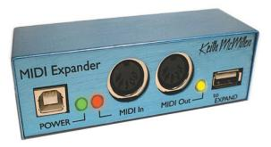
The KMI MIDI Expander is an optional accessory, which enables use of QuNexus with hardware MIDI devices. Plug the receiving MIDI device into the MIDI Out port and QuNexus will send MIDI data through a regular 5-pin MIDI cable.
