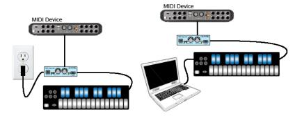
The KMI MIDI Expander is required to send and receive MIDI Data via 5-pin MIDI devices. The MIDI Expander can be used with or without a computer or iPad connected. Power is supplied to QuNexus from the MIDI Expander's power port when the MIDI Expander is plugged into a power outlet. If connected to a computer (or iPad) and a MIDI Expander, power is supplied to the QuNexus from the Micro USB port instead of the Expander.
