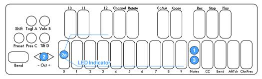
To **Transpose** the QuNexus, use the key labeled "Xpose" with the steps listed above. You can go up or down 11 semitones. If you are below 0 the - Oct button will blink; if you are above 0 the + Oct button will blink.
