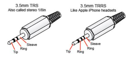
These are the 2 types of plugs that are required to plug QuNexus into a CV device. The TRS type is for the CV output ports and the TRRS type is for the CV input port.
