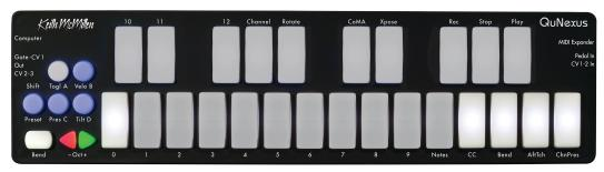
These key buttons act as toggles as well to turn Channel Pressure, Poly After Touch, CCs, and Channel Rotation on and off. Note that if you turn CCs off, all 3 possible CCs from Keyboard Layer will not output unless you turn them back on.
