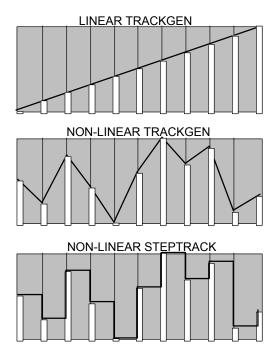
TIP: The Tracking Generator can be used to turn a variable control, such as the Mod Wheel or velocity, into a switch by setting all of the points to 0 except for point 10. Only near the maximum input will anything other than 0 come out of the Tracking generator.
