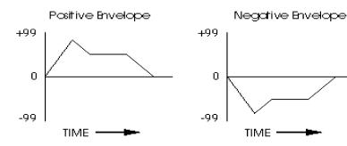
NOTE: Pitch Envelope parameters (such as attack and decay time) are programmed within the Pitch Envelope Function on button [90].
