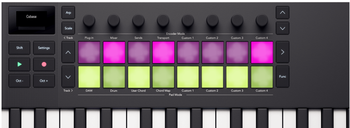
The Launchkey Mini 37 pads reflecting the mixer Mute and Solo states on the pads.
